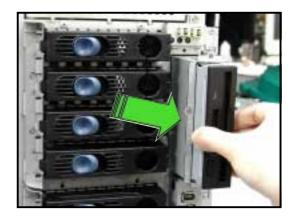
3. Disconnect the floppy disk cable and power cable from the drive to completely release the drive.
